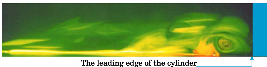
Fig. 6. Side view of the turbulent junction flow ahead of the square cylinder at Re = 32,000 .
